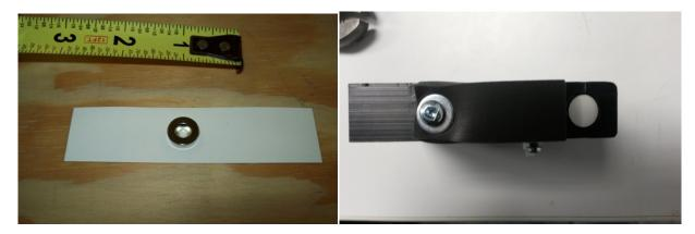
This magnet must be aligned with the sensor in the shelf rest.
