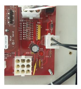
Step 4– set you meter to Ohms ( $\Omega$ ) in the lowest setting (typically 200) and insert a probe into each pin
