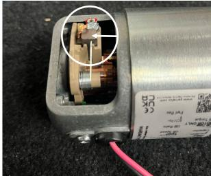
With your finger, push the motor brush back in. The spring should hold the motor brush firmly in the mount.
