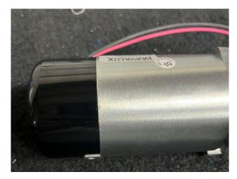
You will see on each side the motor brush is held in by a spring. This motor brush has ejected from the mount.
