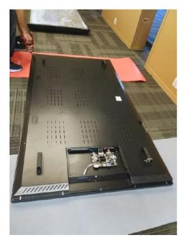
Once on its front, 24 screws will need to be removed from around the perimeter of the display, as well as an additional 16 screws from around each of the VESA mounting positions and 7 screws removed from an access panel for the AD board, note: bolts are hand tightened and can be removed without a tool:
