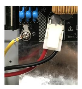
Use a flat blade screw driver to depress the two exposed locking tabs on the power receptacle and push towards the outer edge of the monitor. There are two more locking tabs on the opposite side of the receptacle depressing those will allow the receptacle to be completely removed from the metal monitor housing.
