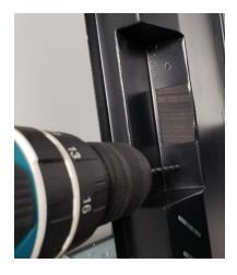
Remove all metal shavings from the drilled holes, insert the socket into the hole in the monitor housing, insert the included 6/32 Pem studs though the holes drilled previously and secure on the inside of the housing using the supplied 6/32 lock nuts.
