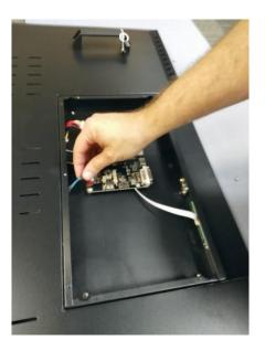
Lift the back cover of the monitor from the top edge (opposite of power cord receptacle) being careful not to pull the wiring connecting the power supply board and the receptacle. Unplug CON 1 from the power supply board and remove the screw holding the yellow/ green wire from the power supply mounting panel
