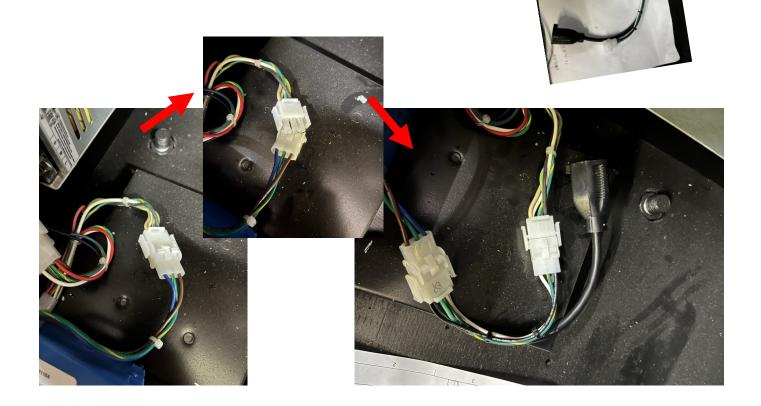
**Step 4:**Push the tab to release the AC prongs and replace with USA Prong.
