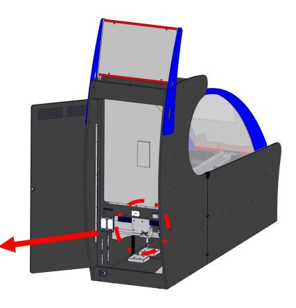
**Step 2:**Cut the red wire flush to the connector.
