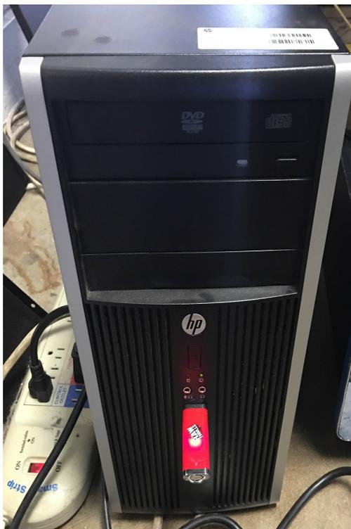
Plug the flash drive into the PC you wish to update. Then power-cycle the machine.
