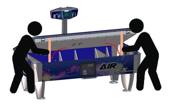
With a third person, remove the pins on the gas shocks. To do this, flip the pin around and slide it down and out the hole. Then pull the gas shock off the anchor and lay on the ground. Now close the top.
