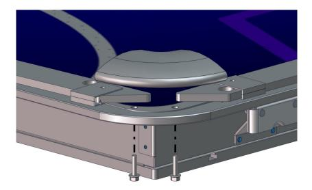
Lift the playfield out. Replace with new playfield. Assembly in reverse. Please note on last page the layout for the ball deflectors proper placement.
