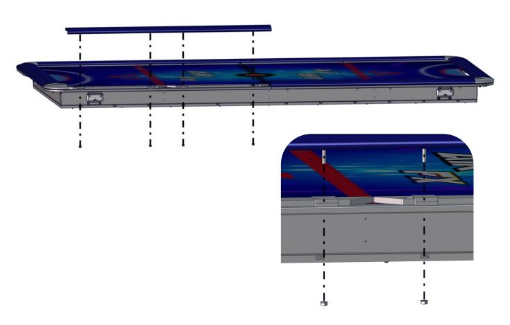
Remove all corner rails. To do so, remove the two bolts holding the corner Repeat this all the way around the playfield.
