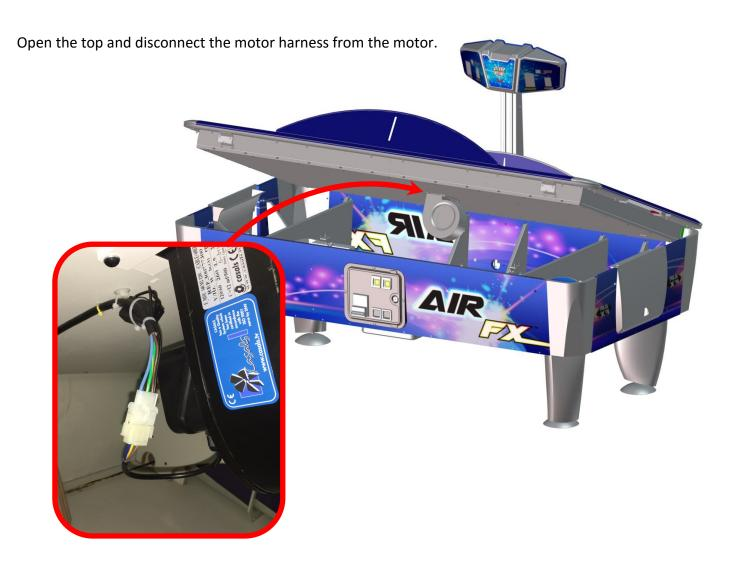
Then remove the four bolts holding the blower motor to the playfield and put aside.
