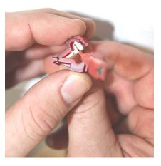
Connect the Freeplay Button Orange Wire to the T-Splice.
