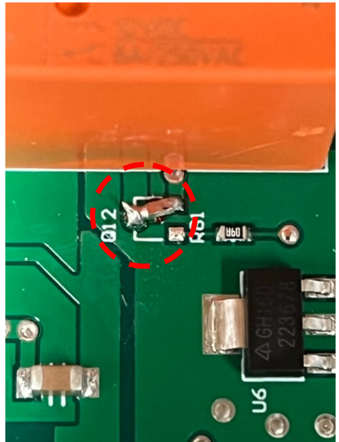
0 ohm resistor installed in place of Q12 transistor.
