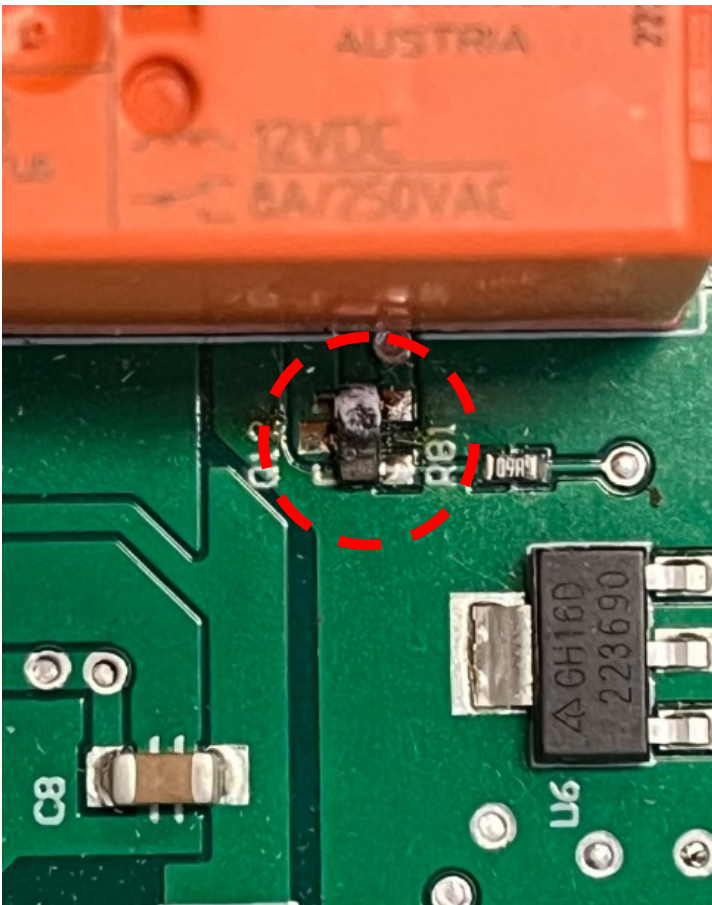
Failed component at Q12. This controls the ball gate.
