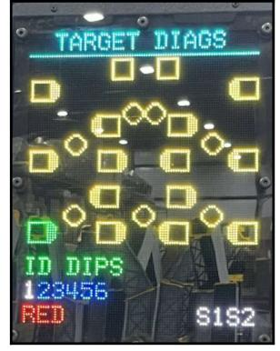
You will also notice the numbers under "ID DIPS". This indicates the proper dip switch setting for this location. IT IS NOT READING THE DIPSWITCHES! It is only showing you the proper settings for that location. White means it should be set to on while blue means it should be set to off.
