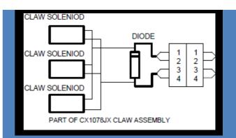
The claw coils measure 18 Ohms each. Wired together in parallel, the resistance across the circular plug is 6 Ohms. Be sure to measure across pins 1& 4 and 3& 2.
