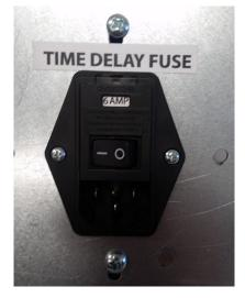
3) using a small flat blade screw driver open the fuse access door
