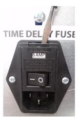
4) use a flat blade screw driver to remove the fuse cartridge.
