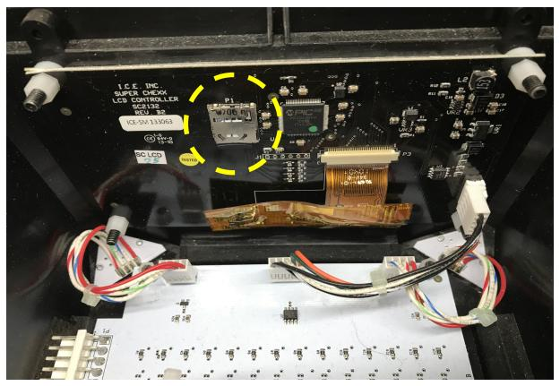
On each display there is a micro SD card connector. Push the card in lightly until it clicks and let go. The card should pop out slightly. With your nail pull it out. Insert the new card the same way the old card was. Push until it clicks. The card will remain in the connector.
