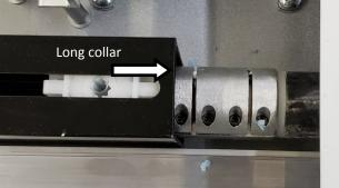
Using a 1/4 inch driver (or a multi screw driver) and the supplied No. 1 square bit in the parts kit tighten the screws so the rod and gear box so they hold together.
