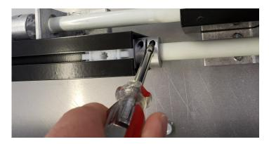
PLAYER ROD & GEAR BOX SHAFT MUST MEET IN CENTER OF COLLAR SLOT
