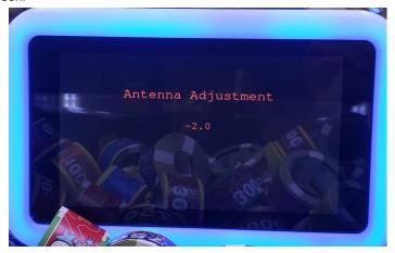
4) using the up and down arrows adjust the value for the antenna adjustment, the range is between -3.25 to 5.25. Once the desired value has been set press "t" on the keyboard to save and exit, unplug the USB keyboard and reconnect the USB connection to the main board.
