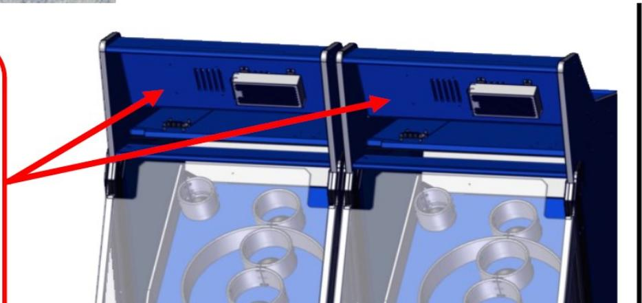
Step 6 - check the interconnect phone lines that run between the game are connected to the led driver board located behind the display.
