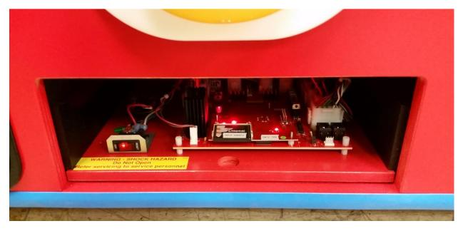
Inside the game you will see the bottom of the pan that the balls roll down. Mounted to that pan is the safety sensor
