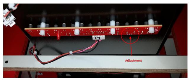
There is an indicator led on the sensor, normal operation when the game is in attract mode the LED will be flashing, when you coin the game up the led will go off and then when you block the sensor the led will turn on. There is an adjustment for the sensitivity of the sensor. It is located along the back edge of sensor to the right of the connector. Turing the adjustment all the way towards the connector will set it to the least sensitive position.
