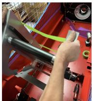
**Step 13:**Loosen on both side the top adjusters using a #2 Phillips screw driver. DO NOT REMOVE!
