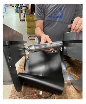
The roller with the abrasive material goes at the bottom while the smooth roller is installed at the top. Notice the center groove in both rollers. When installing the new belt, the belt has a matching groove that must be installed into these grooves.
