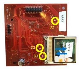
**Step 1:** Reseat Compact Flash card — With the power off, pull out the compact flash card and then push it back in. Turn power back on.
