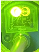
When unblocked and aligned, they will have both green and yellow LEDs on.
