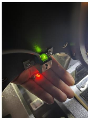
If LEDs work as described, measure the voltage coming out of the sensor. Gray/violet is the output, orange is +12 and black is ground. Be careful, the sensor has black as its output and blue as the ground. A proper sensor will measure .5 VDC when blocked, +12 VDC when not blocked.
