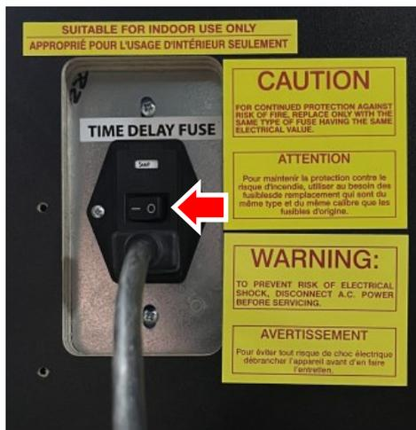
If the switch is on, verify the time delay fuse. To do this unplug the AC cord. Do not proceed with the AC cord plugged in!
