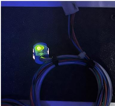
Blocked or reflector is misaligned or missing.
