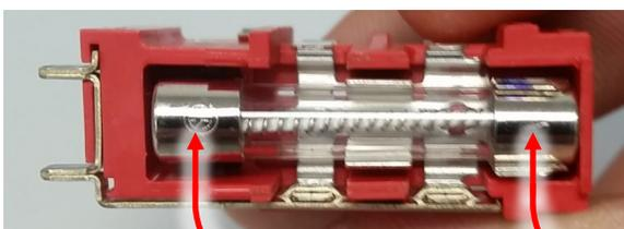
In most cases, the fuse will have a burnt mark in the center but it is always better to measure the ohms between the ends of the fuse. It should measure below a ohm. Anything more, replace the fuse. If still more than an ohm, replace the power module.
