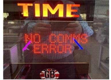
**Step 1:** Confirm both the main board and bottom back display board has power.
