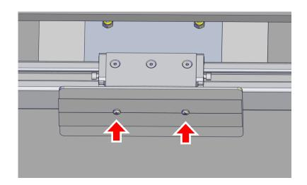
**Step 6:** Install the new reflector using the previous hardware.
