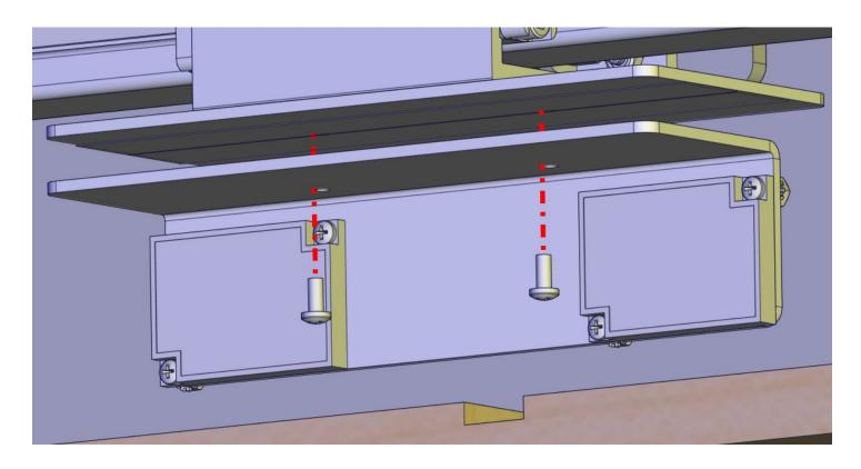
**Step 7:** Install the sensor bracket using the provide AA0655 screws using the provided right angle screwdriver and Allen Bit. Note, sensor points at the reflector, not toward you!
