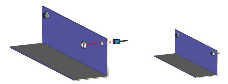
**Step 5:** Remove the old reflector mounted under the slider using the provided right angle screwdriver and Phillips bit.
