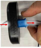
**Step 4:** Insert the sensors as shown and use a plastic nut to secure them to the bracket.
