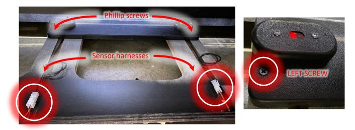
**Step 3:** Remove the two Phillips screws holding the sensor plate to the sensor platform. Once the sensor housing is free, gently push the sensor from the front of the housing as you pull slightly from the rear. Make note of how the sensor is seated in the housing, you'll want to make sure the new sensor is flush once re-inserted into the housing.
