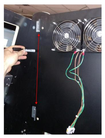
4.) Align the power assembly left of the line you drew. So that when the wood is installed the power assembly doesn't interfere with mounting. It's a tight fit you have to go higher than the screw with the chain on it (red arrow), high enough so the monitor power supply isn't in the way of the upper left hand screw (yellow arrow), but not too high so that the panel with the fans on it won't fit on properly (blue arrow) it is hard to see the line drawn in the picture.
