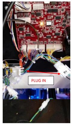
8.) Unplug connector P2 on the board and plug in the new connector that goes up to the power supply that you just installed. You can take out the old harness P2 that goes to the computer, or you can leave it in the game unplugged it doesn't matter either way.
