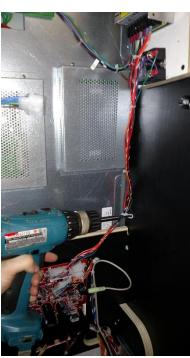
6.) Unplug the connector that says Monitor, and plug in the connector that goes to the power supply you just installed.
