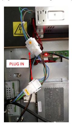
7.) Unplug the harness that says PC down by the red board. And plug in the connectors at the end on the longer brown and black wires.
