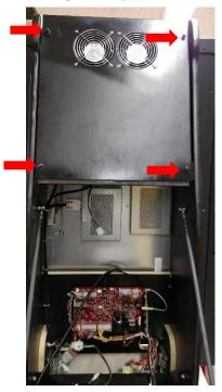
3.) Take the panel and hold it to the two metal brackets that held it on the right hand side. Take a marker and draw yourself a reference line from bracket to bracket.
