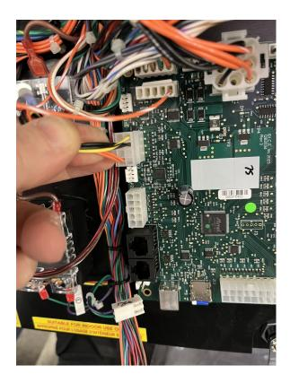
**STEP 6:** Remove P1 and P3 by pinching the lock tab at the top, then pull straight out. The lock tab prevents the harness from coming out.
