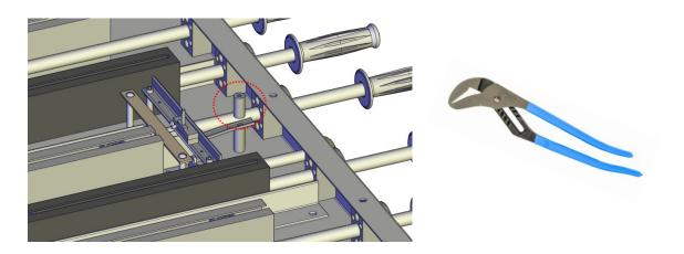
**Step 8:** Remove the Phillip screw located at the opposite end of the chute (it is surrounded by a wall, a magnetic screw driver is suggested.
