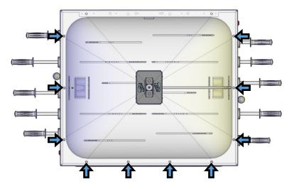
**Step 1:** Open the dome by removing all the bolts around the dome.
