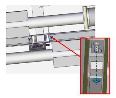
**Step 9:** Remove ramp and flip ramp over. If you see a line stamped into the metal on the small hole side, the ramp is defective and requires replacing. Please contact our parts department to obtain the replacement. A photo and the defective part is required to claim warranty.
